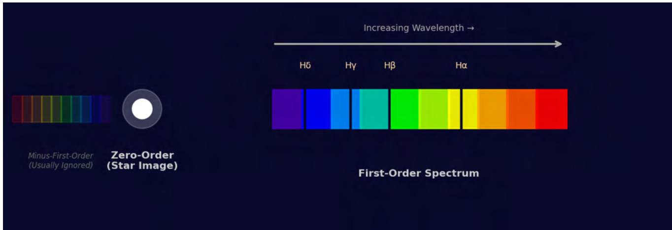
Figure 2: Illustration of what you see on the camera sensor after installing the diffraction grating. The bright zero-order image (the star itself) appears alongside the first-order spectrum, which shows the dispersed light with visible absorption lines (Balmer series in this case). The faint minus-first-order spectrum on the opposite side, if observed, is typically ignored.
