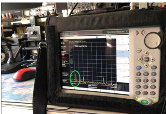
Image VIII: visualization of possible solar flare with a spectrum analyzer and a 40-m triangular loop (February, 2025)
